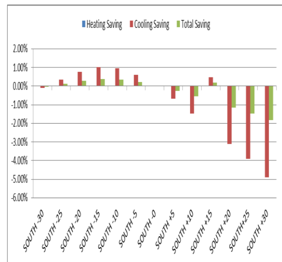
Figure 15 The energy saving in exact directions angle between (150-210) of Cylindrical Shell
