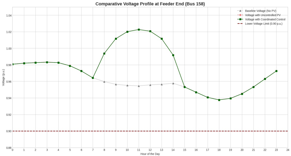
Figure 7 Impact of PV integration and control on the end-of-line voltage.
