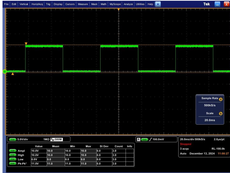
Figure 2 Gate Signal Supplied to MOSFET During Tests
