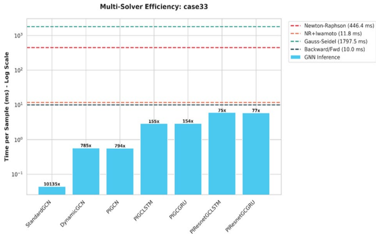
Figure 18 Efficiency analysis the proposed Graph Neural Network models across the IEEE 33-bus systems
