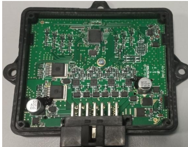
Figure 3 L9963E Data acquisition module
