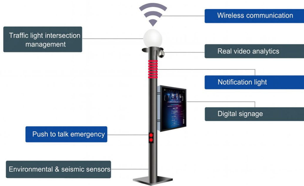
Figure 5 LED-based smart street lighting pole system and its components
